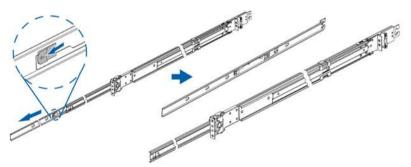
2 Middle rail within the rail return. Press this part in the direction of the arrow back in the middle rail.
