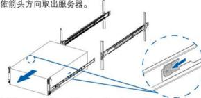
4 Off shrapnel taken out of the rail in the direction of the arrow. 拉开弹片依箭头方向取出内轨。
